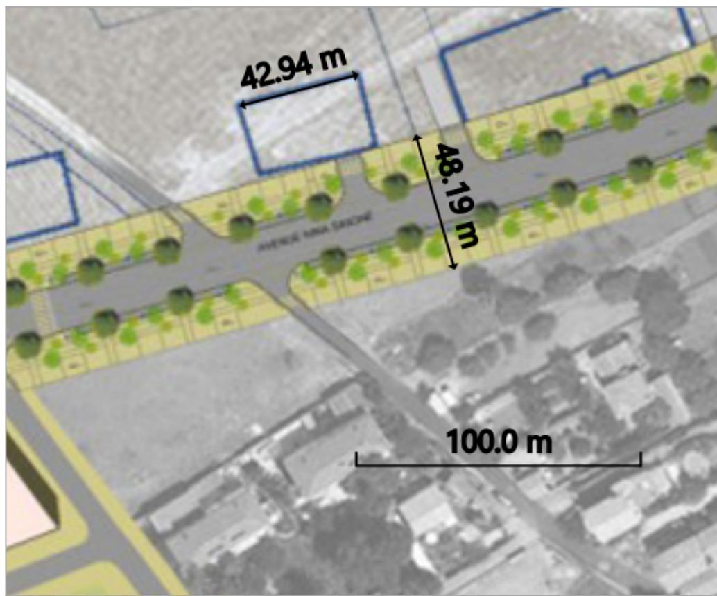
In this example, we realize that the scale is wrong, because the track is actually much less than 48 m wide.
