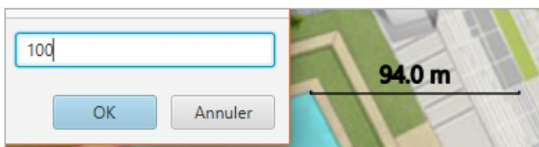
The scale is redimensioned and can now be moved wherever you want on the map. The length of the end returns of the scale is specified by right-clicking > **Properties** > then setting the **Border height** :
