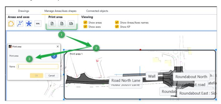
Once the print area zone is named, it appears on the *Drawings and phases* tab in the list of drawings:
